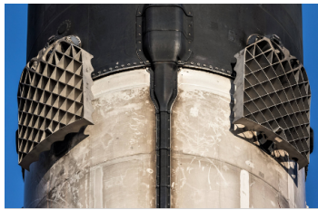
Figure 2: Burned Grid Fin of Falcon 9
